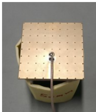
Ground above antenna
