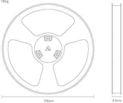
12000 pc LLP.2450.X.A.30 2 reel in small inner box Dimensions - 190\*190\*28 Weight - 0.42Kg
