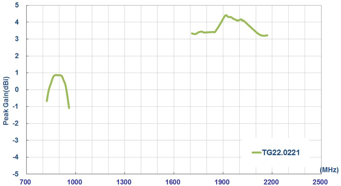
Figure 4. Peak Gain of the TG.22 Antenna.
