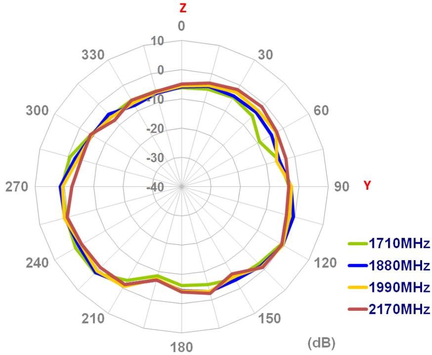
**Figure 6.** 2D Radiation Pattern of the TG.22 Antenna.
