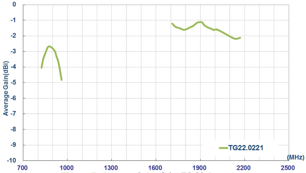
**Figure 5.** Average Gain of the TG.22 Antenna.
