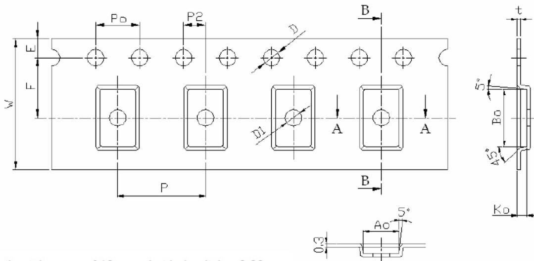
1. Cumulative tolerance of 10 sprocket hole pitch:  $\pm 0.20\text{mm}$
