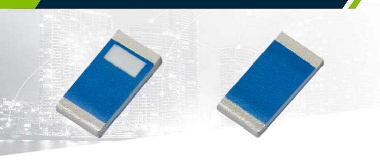
The WLA.10 2.4 / 5.8 GHz Loop antenna is a high efficiency, miniature SMD, edge mounted ceramic antenna for Dual-band 2.4 / 5.8 GHz Wi-Fi and 802.11 applications where PCB space is limited, such as hand-held devices. The WLA.10 uses the main PCB as its ground plane, thereby maintaining good efficiency despite its small size. The efficiency is very stable on the complete bandwidth of both lower and upper bands allowing for maximum data throughput rates on all channels available.
