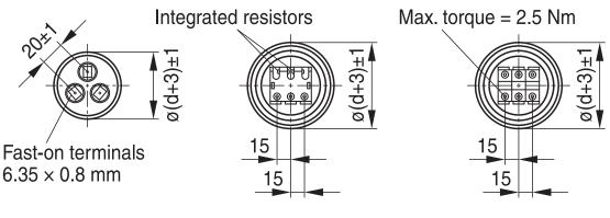
Creepage distance > 12.7 mm Distance in air > 10 mm KLK1857-M-E
