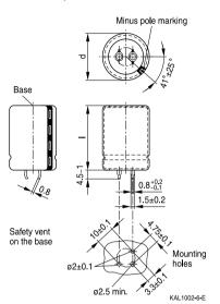
Snap-in terminals, length  $(6.3 \pm 1)$  mm. Also available in a shorter version with a length of (4.5 - 1) mm. PET insulation is marked with label "PET" on the sleeve.
