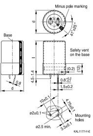
Snap-in terminals, length (6.3 + 1/-1.4) mm. Also available in a shorter version with a length of (4.5 - 1.4) mm. PET insulation cap is positioned under the insulation sleeve.
