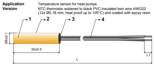
$L = 870 \pm 10 \text{ mm}$  $L1 = 4 \pm 1 \text{ mm}$  dimensions in mm
