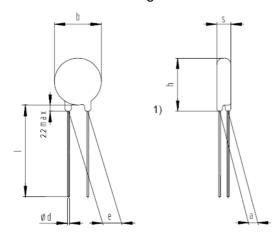
$b_{\text{max}}$ 9.0  $h_{\text{max}}$ 11.0 = 3.6  $\textbf{S}_{\text{max}}$  $5.0 \pm 1.0$ е = 1.2  $a_{typ}$ = 29.0±2.0 =  $\varnothing \mathsf{d}$  $0.6 \pm 0.05$
