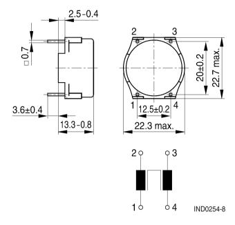
Tolerances to ISO 2768-cl / ISO 8015. Size ISO 14405 (E) All dimensions in mm
