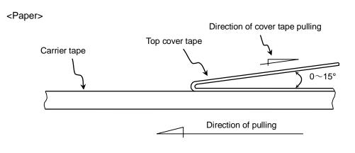
Paper tape should not adhere to top cover tape when pull the cover tape.
