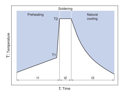
Natural cooling Preheating Peak Time Temp. Time Temp. Time t1 T2 t2 t3 110°C min. 30 to 60s. 260°C Within 10s. Over 60s.
