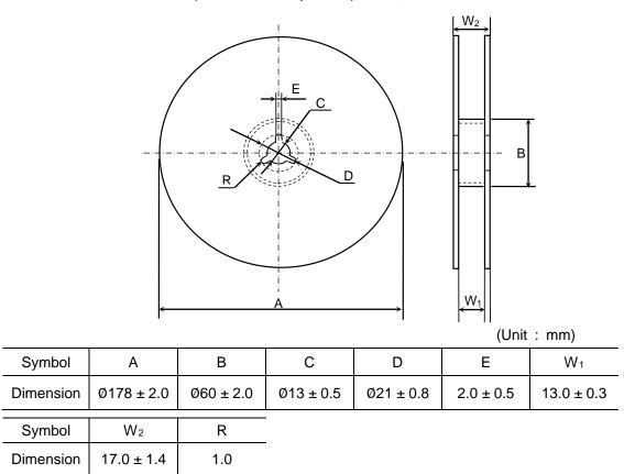
Dimensions of reel (Material : Polystyrene) CGA1, CGA2, CGA3, CGA4, CGA5, CGA6
