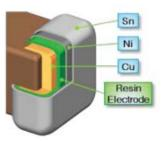
conductive resin layer to the end terminal electrodes. This allows the capacitor to better absorb mechanical stress, while TDK's superior layer bonding technique reduces the risk of separation failure. Designers who are specifically concerned with mechanical stress or who have had issues in the past with capacitor cracking should look to TDK's C Series Mid Voltage Soft Termination MLCCs.
