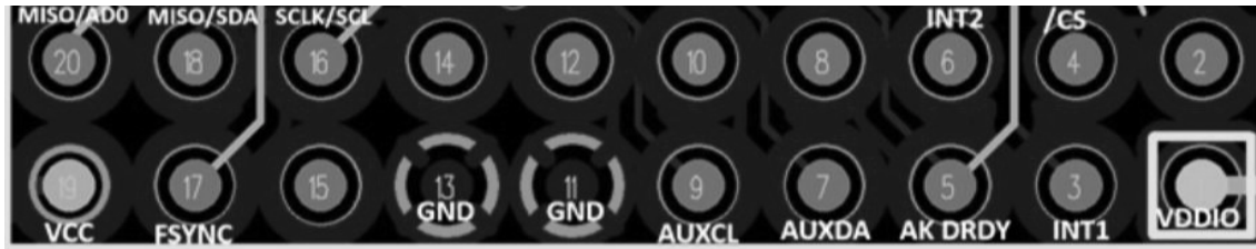
Figure 4. Pin out of CN1 (Connector to EVB)
