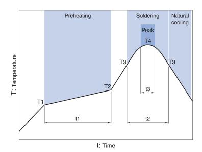
Preheating Soldering Peak Temp. Temp. Temp. Time Time Time T1 T2 T4 t3 Т3 150°C 180°C 60 to 120s 230°C 30 to 60s 250 to 260°C 10s max.
