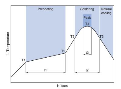
Preheating Soldering Peak Temp. Temp. Time Temp. Time Time **T1 T2** t1 Т3 t2 **T**4 t3 150°C 180°C 90 to 120s 40s 230°C 255°C 10s max.
