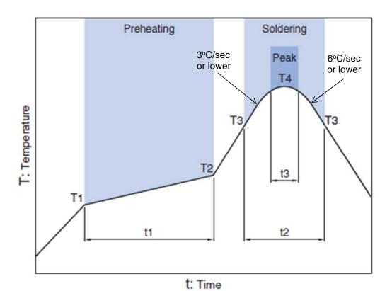
Soldering **Preheating** Critical zone (T3 to T4) Peak Time Temp. **Time** Temp. Time Temp. t1 **T3** t2 **T4** t3 \* T1 **T2** 150°C 200°C 60 to 120sec 217°C 60 to 120sec 240 to 260°C 30 sec Max
