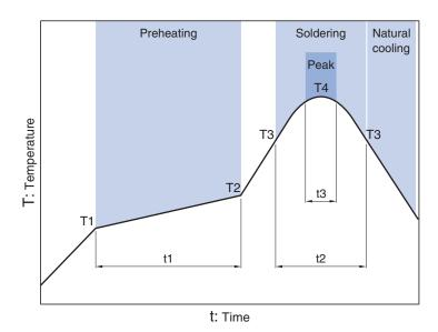
Soldering Preheating Peak Time Time Temp. Time Temp. Temp. T2 T3 T4 t3 150°C 180°C 60 to 120s 230°C 30s 260°C 10s
