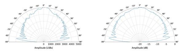
Figure 7. Beam pattern measurements of module in 100 mm plate (raw linear LSB units left, normalized dB right)
