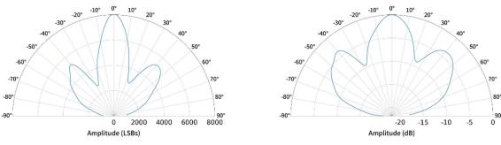
Figure 8. Beam pattern measurements of bare module (raw linear LSB units left, normalized dB right)
