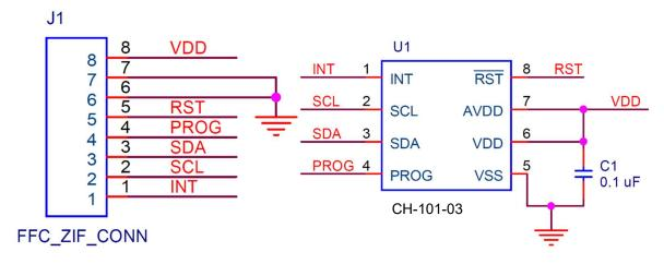
Figure 3. Flat cable connector pin layout (left) and CH-101 board layout (right)
