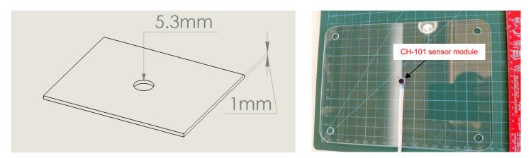
Figure 6. Recommended MOD\_CH101-03-01 module mounting
