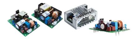
The CUS30M and CUS60M are 2" x 3" footprint AC/DC power supplies with outputs ranging from 5V to 48V. They are certified to IEC60601-1 3rd edition (medical), IEC60950-1, IEC62368-1 and IEC60335-1 with compliance to EN60601-1-2:2015 Edition 4 immunity requirements. Rated at 30W and 60W, these compact products meet class B conducted and radiated EMI in either a Class I or Class II (double insulated) construction, without the need for external filtering.
