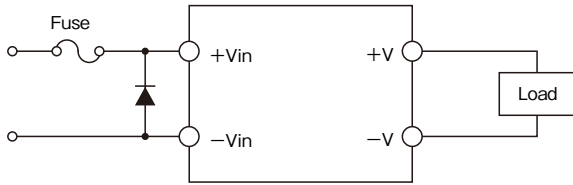
Figure1-5 Protection for Reversed Connection of Input
