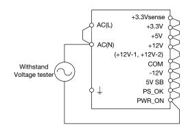
Input - \( \protective earth \) : 2.0kVAC 1min (20mA)
