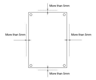
Please leave 5mm space from the surfaces and left 5mm space from the sides of PCB, especially from the solder surface, 8mm space is necessary.
