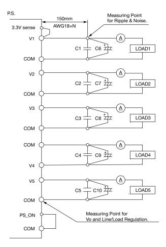
Measure with JEITA RC-9131 probe. Bandwidth of scope : 100MHz
