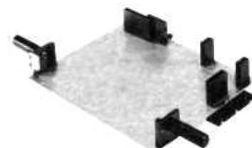
5. Press handle down gently and insert connector into the board.
