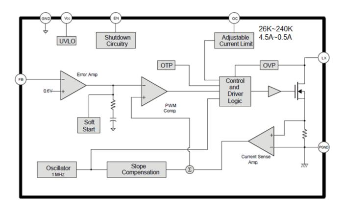
Figure 3 Function Block Diagram of TD8228
