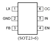
Figure 2 Pin Configuration of TD8228(Top View)
