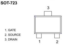
Marking RK \* Or RK \* =wafer tracking no
