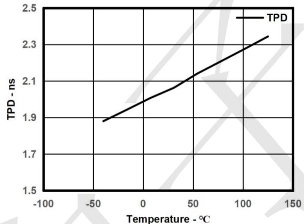
Figure 2. Typical Tpd vs Temp
