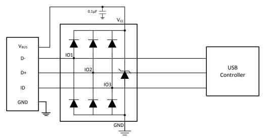
Figure 3. Typical Application Schematic
