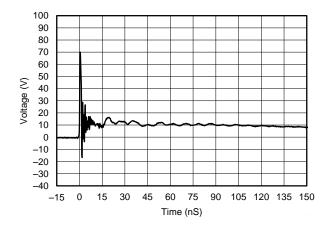
Figure 4. TPD3E001 +8kV Contact IEC61000-4-2 Voltage Clamping Waveform
