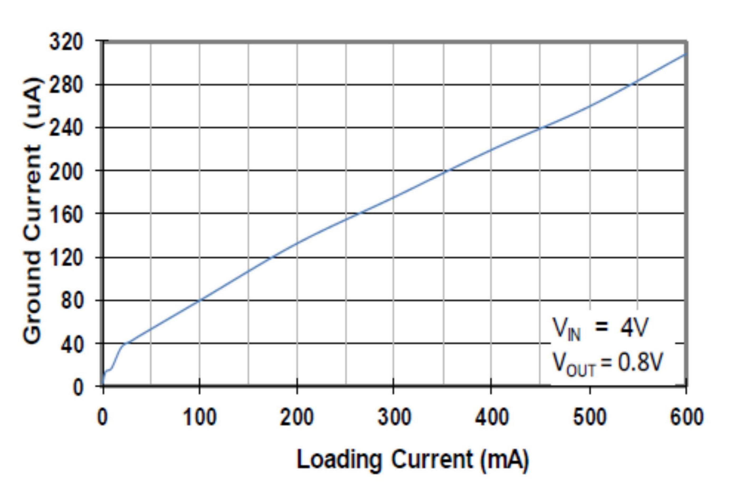
Fig. 10 Ground Current vs. Loading Current
