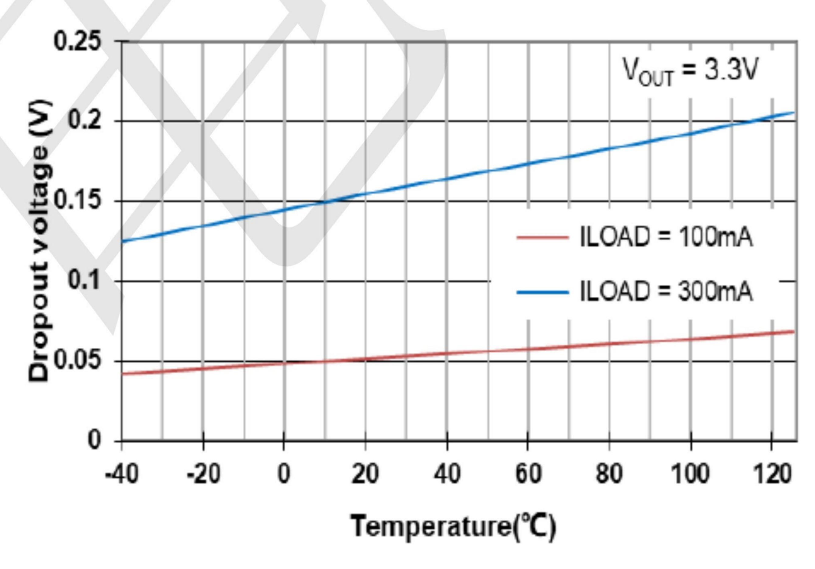
Fig. 8 Dropout Voltage vs. Temperature
