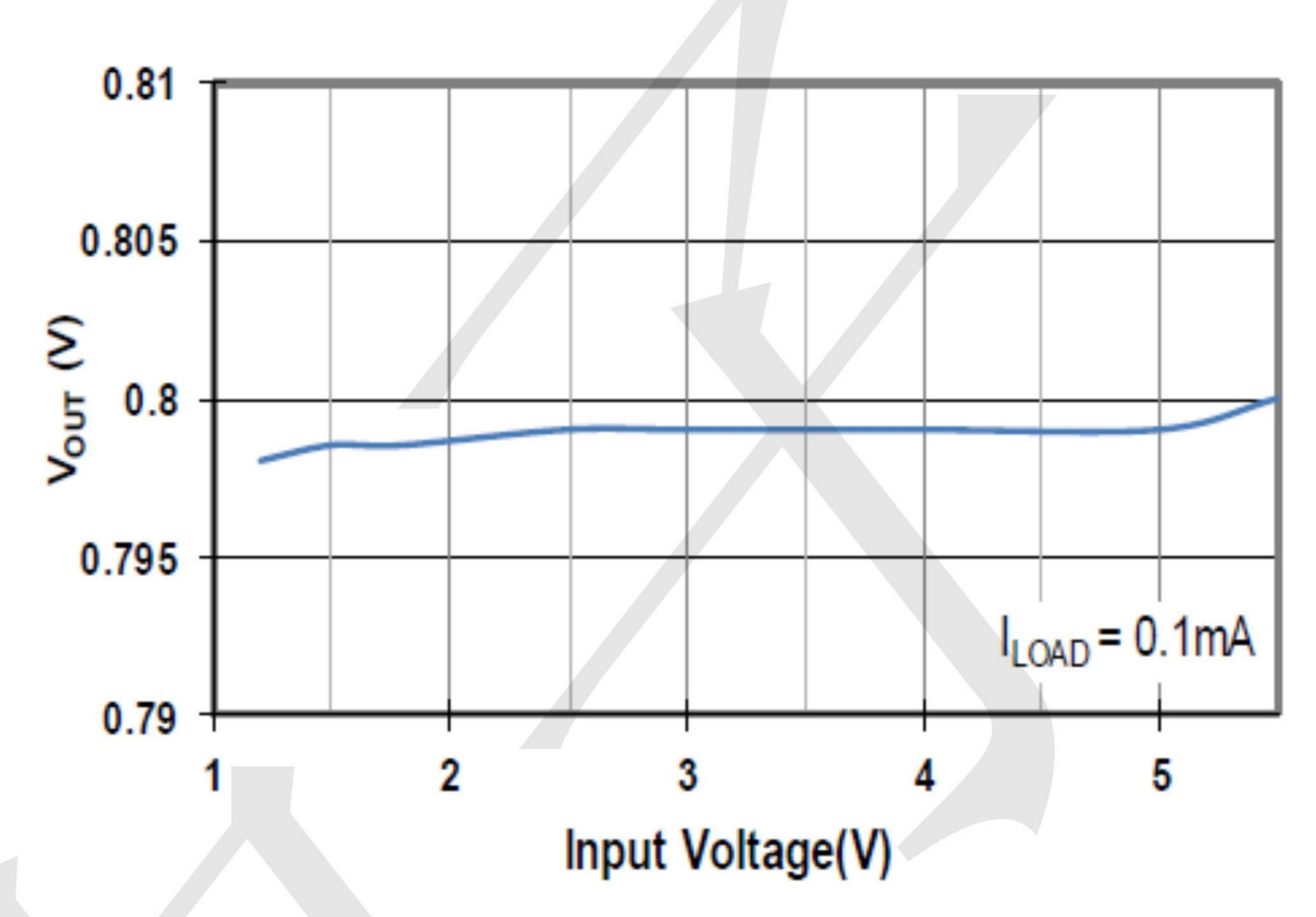
Fig. 6 Output Voltage vs. Input Voltage
