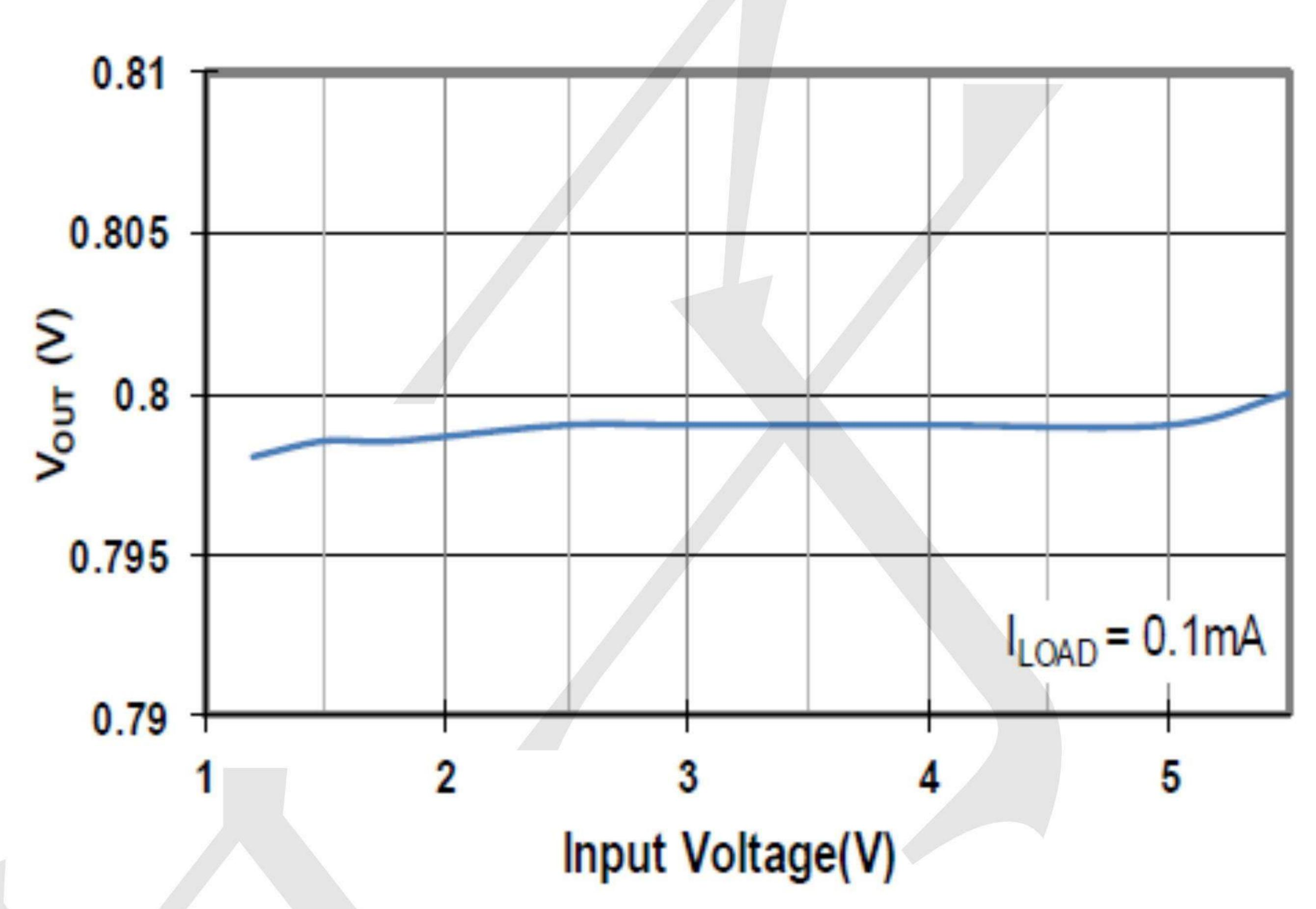
Fig. 6 Output Voltage vs. Input Voltage
