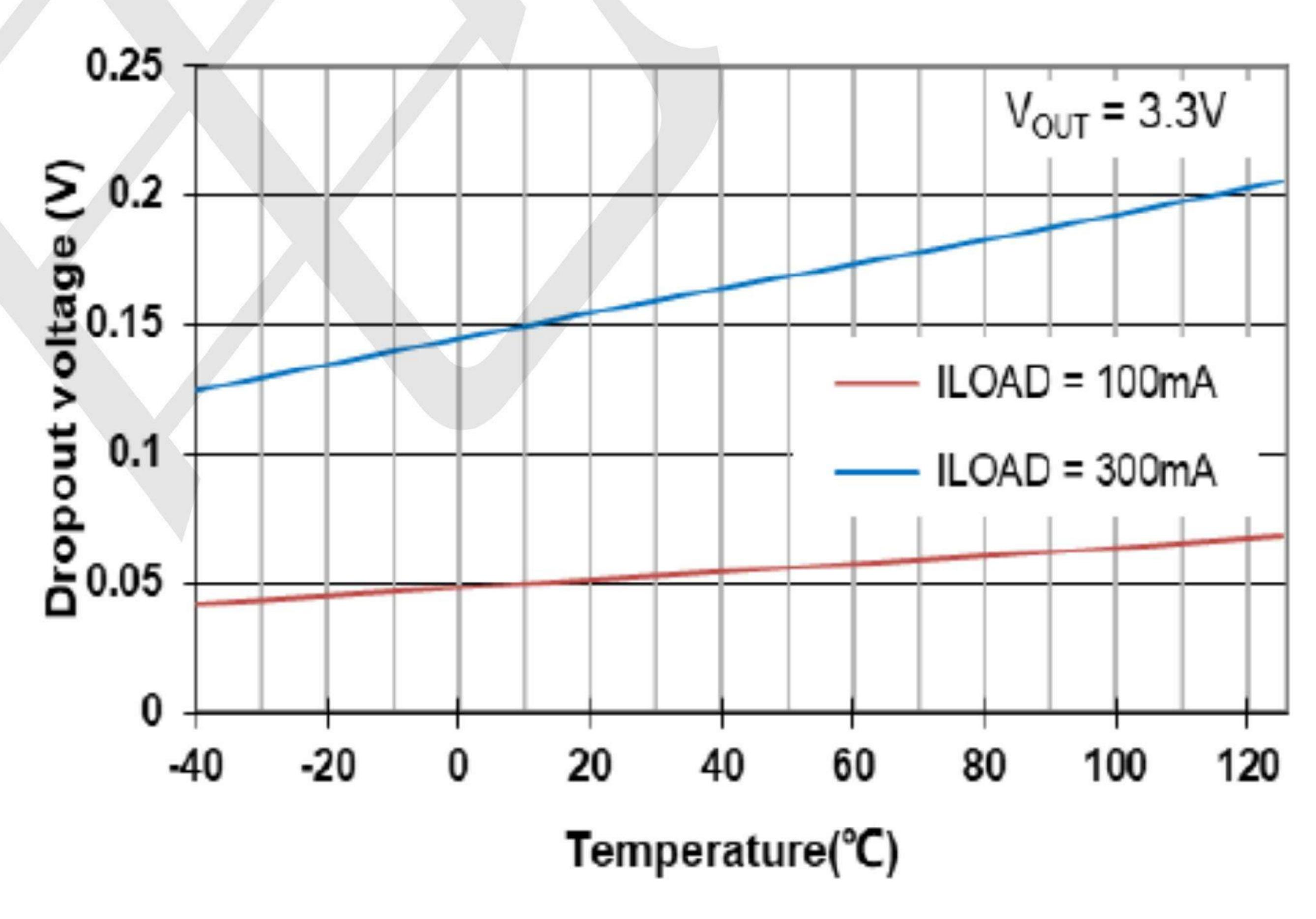
Fig. 8 Dropout Voltage vs. Temperature
