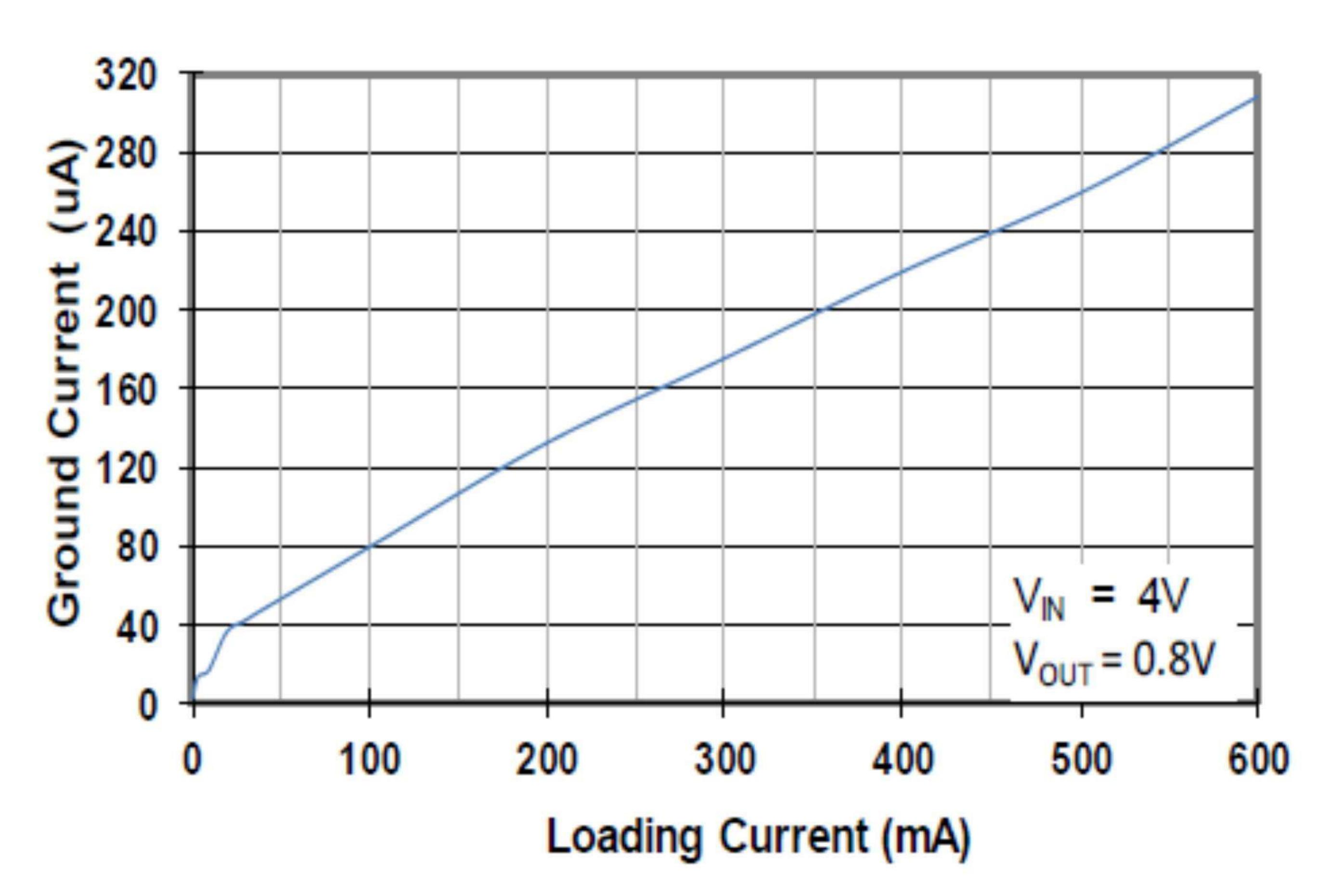
Fig. 10 Ground Current vs. Loading Current
