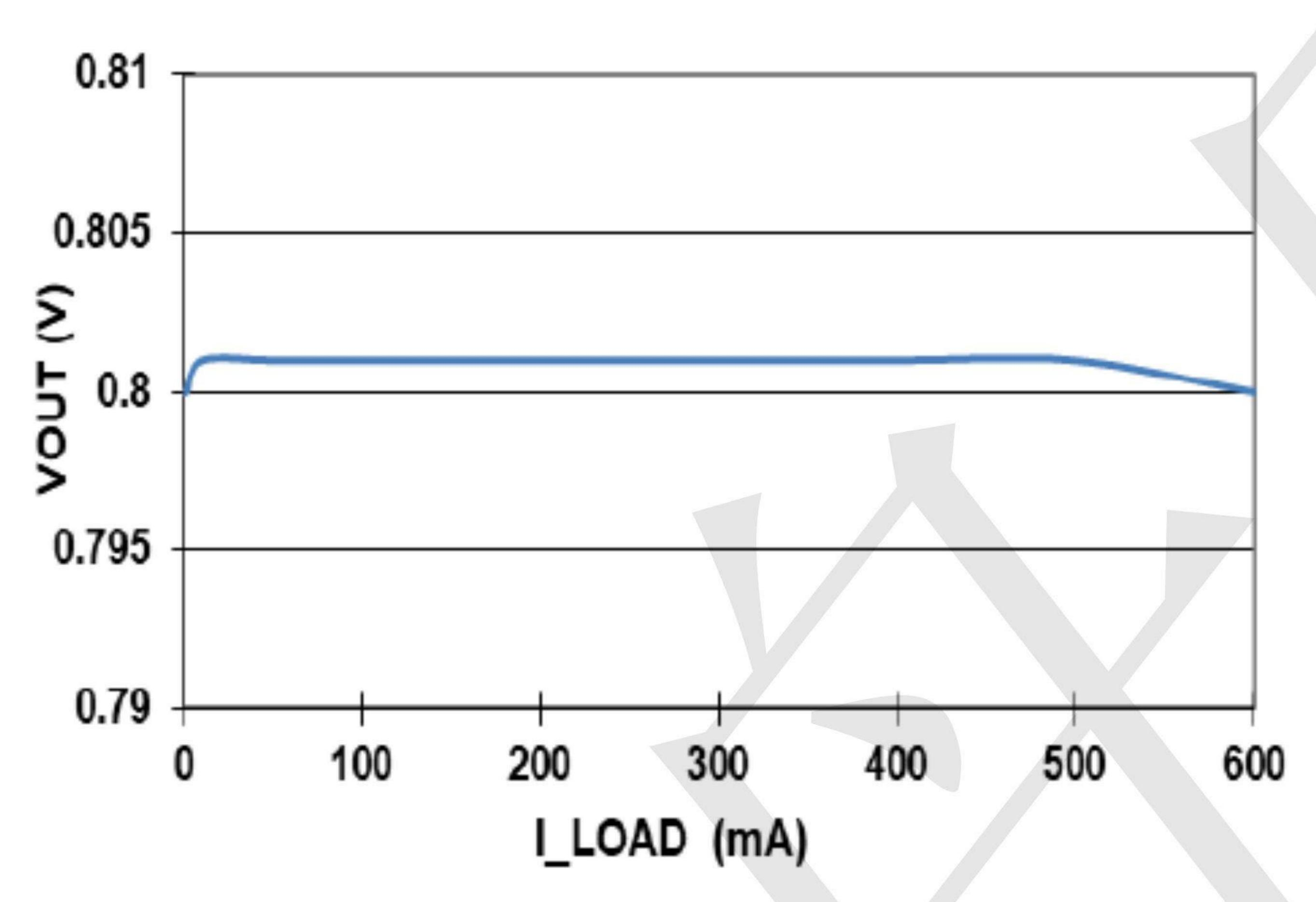
Fig. 7 Output Voltage vs. Load Current
