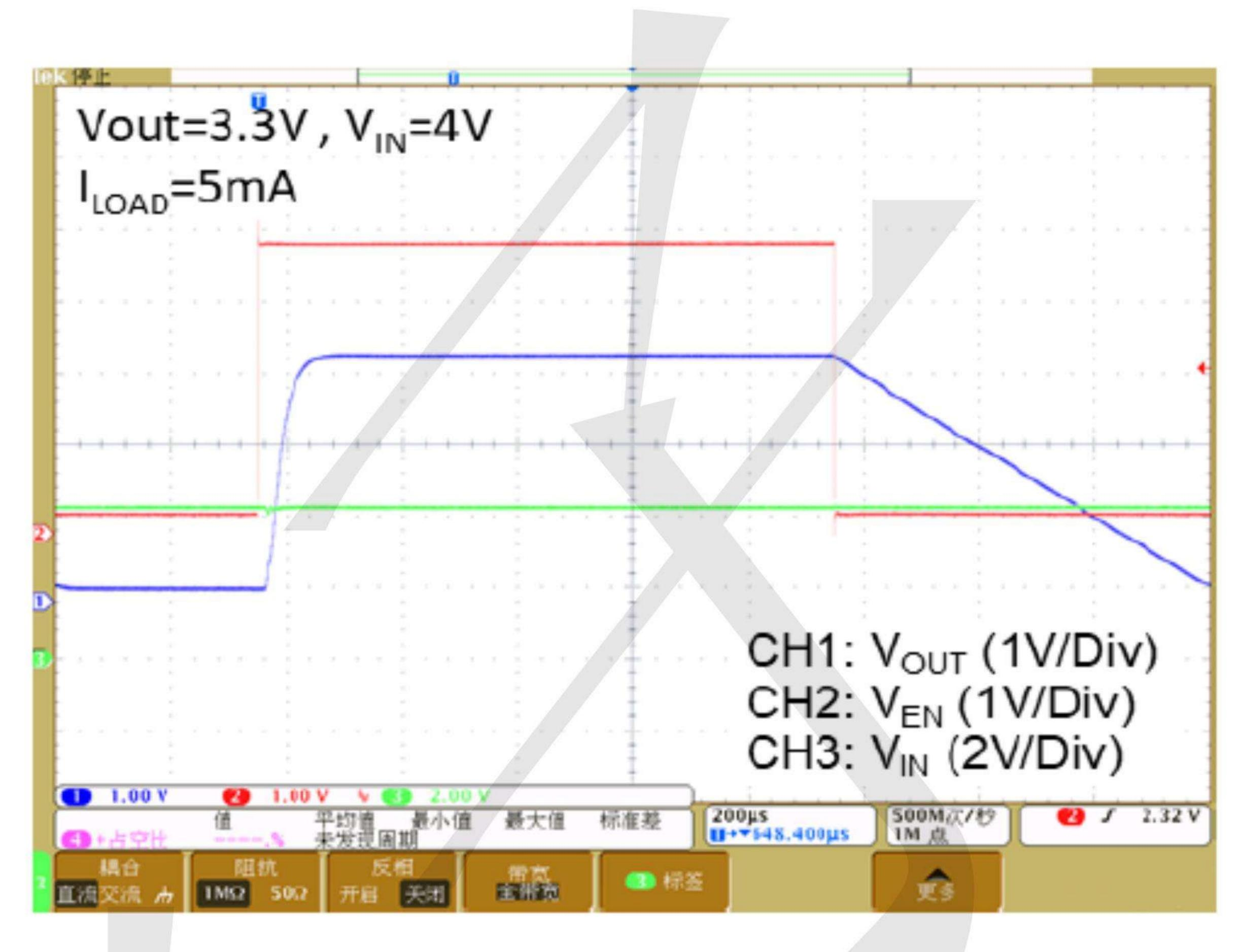
Fig. 18 V<sub>OUT</sub> Turn On/Off by EN
