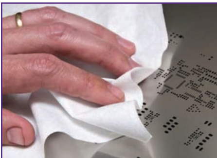
High saturation and snag resistant material ideal for stencil cleaning
