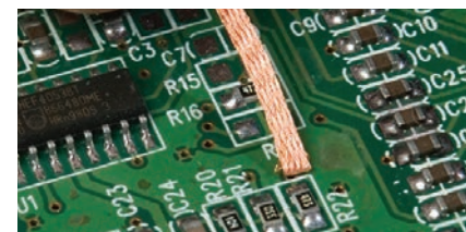
Match braid width to contact area
