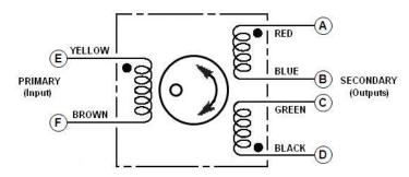
A through F: Connector pin assignments; Connect B to C for differential output
