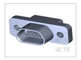
Connector Style: Plug Connector System: Cable-to-Board Number of Positions: 51 Centerline (Pitch): 1.27 mm [.05 in ] Connector & Contact Terminates To: Wire & Cable
