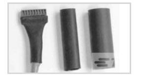
Primary Product Color: **Red** Wall Type: **Dual** Expanded Inside Diameter (Min): **19.1 mm [.75 in ]** Recovered Inside Diameter (Max): **6 mm [.23 in ]** Shrink Ratio: **3:1**
