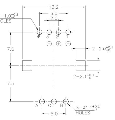
MOUNTING HOLE DETAIL VIEWED FROM MOUNTING SIDE P.C.B t=1.6mm
