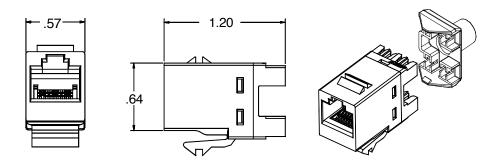
CommScope's Category 6 SL series modular jacks exceed ANSI/TIA-568-C.2 and ISO/ IEC 11801 component requirements and Category 6/Class E system performance. CommScope's Category 6 System complies with all of the performance requirements for current and proposed applications such as Gigabit Ethernet (1000BASE-TX), 10 and 1 OOBASE-TX, loken ring, 155 Mbps ATM, 100 Mbps TP-PMD, ISDN, analog and digital video, and analog and digital voice (VoIP).
