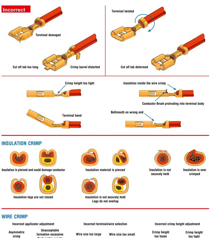
**Terminal feed** incorrectly adjusted flash and/or cracks
