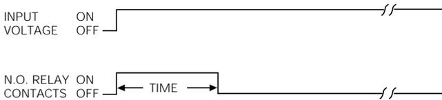
**Interval on (with control switch)** – Input voltage must be applied continuously to operate the internal relay. The relay energizes and timing begins when the external switch is closed. At the end of the time delay period the relay will de-energize. Reset is accomplished by opening and reclosing the control switch.
