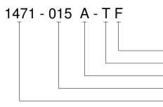
Coating (F = Gel Fill, Blank = No Coating) Port (T = Tube, N = Narrow Hole, W = Wide Hole) Type (A = Absolute, G = Gage) Pressure Range Model
