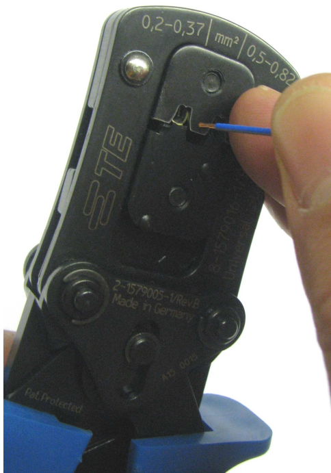
Picture 6: Inserting the stripping wire into the insulation stop
