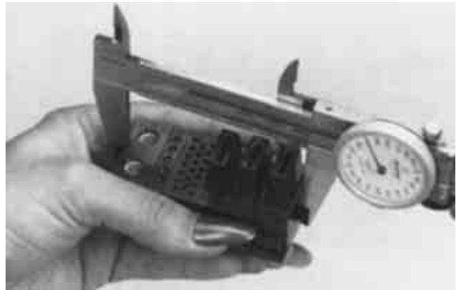
2. Measure length of assembly, and add .100" (2.54 mm) to determine overall rail length. Cut rails to length.
