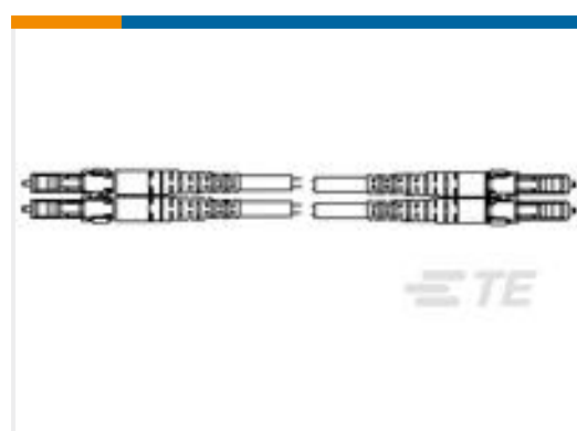
TE Part #2064915-3 C/A,F/O,2F I/O MM50 OM3,SCLC DPX
