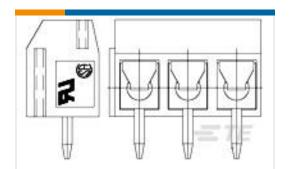
TE Part # 1776244-2 Vert Side Wire Entry, 5.0mm, B TE Part # 1776489-2 Unshrouded Header, 5.0mm, HT, Blue
