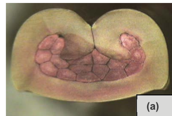
Significant flash can be generated with excessive anvil to crimper clearance, as shown by nominal design condition (a) and +0.003 in over nominal
