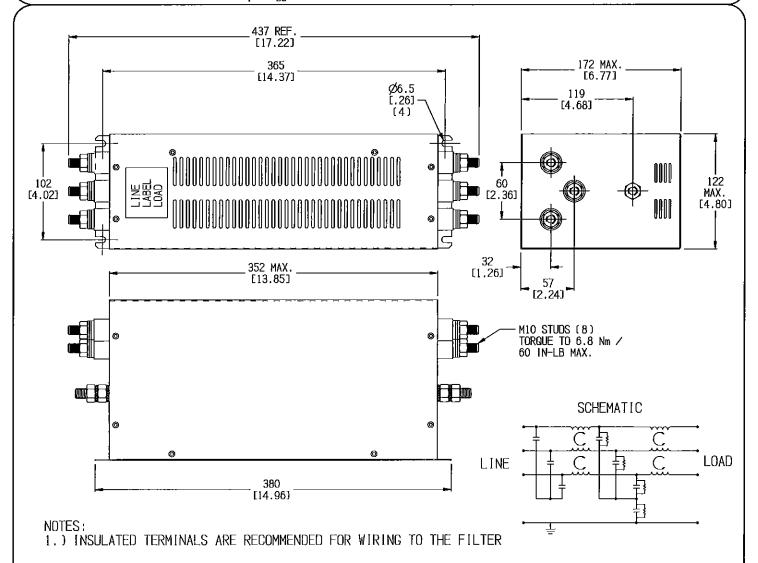
$50 \Omega - 50 \Omega (TYPICAL)$ INSERTION LOSS FREDUCYCY .30 .50 5.0 10 30 .01 .03 .05 . 10 15، 1.0 3.0 COMMON 27 72 29 11 36 49 57 77 61 47 40 15 ďΒ DIFF 27 37 40 50 73 73 60 50 47 42 30 42 佃 THIS INFORMATION IS CONFIDENTIAL AND PROPRIETARY TO TYDO ELECTRONICS DEPROATION AND ITS URLIDVICE SUBSIDIARIES AND AFFILIATES. IT WAY NOT BE DISCUSSED TO AMENDE THEY THAN THE LECTRONICS PRESSAMEL, WITHOUT WRITTEN AUTHORIZATION FROM TYDO ELECTRONICS DEPORATION.
