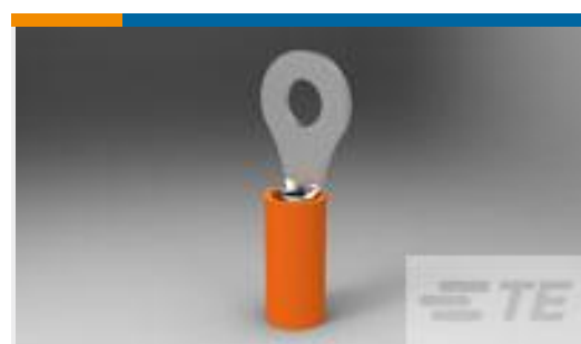
TE Part # 152885 TERM, RING, PIDG, 18-16 AWG, #6, ORNG
