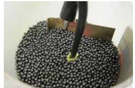
Figure 6 - Dielectric Strength Test - PLASTI-GRIP Terminal
