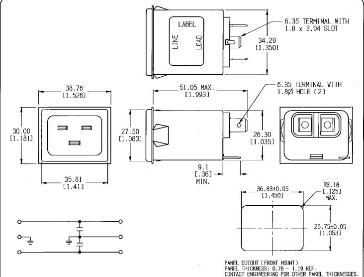
PARTS SHALL COMPLY WITH TYCO ELECTRONICS 138-702 SPECIFICATION FOR HAZARDOUS SUBSTANCES 50 ഫ -50 A (MINIMUM) INSERTION LOSS UNLESS DTHERWISE SPECIFIED TOLERANCE TO BE ±0,64
