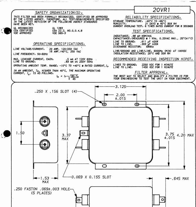
UNLESS OTHERWISE SPECIFIED, 50n 50n (MINIMUM) INSERTION LOSS TOLERANCE TO BE ±.025 FREQUENCY .5 . 15 .3 1 5 2 10 20 30 MHz MATERIAL & FINISH: AS SUPPLIED This document is proprietary to CORCOM INC. and is not to be reproduced nor used for manufacturing purposes except on CORCOM'S prior written consent. COMMON POWER LINE FILTER 11 33 50 65 65 65 62 60 / / 65 ďΒ DATE: 9-15-93 CATALOG NO. DIFF. APPRVD. TAM 15 52 52 65 65 60 20VR1 ď₿ 20VR1.07
